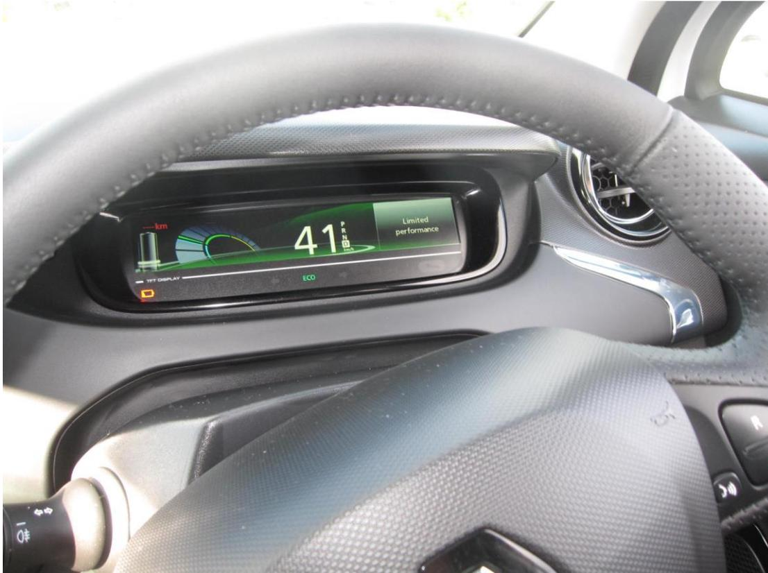
Figure 5: Zoe display showing battery warning lamp, “limit performance” warning and range blanked out
